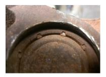
then deform the yokes to secure the bearing cups in position. Therefore, the number of repair shops that are capable restaking u-joints is limited. It is difficult to securely re-stake a bearing cup in a yoke that has been previously staked due to the already deformed yokes and therefore, most staked u-joint axles & driveshafts are not serviced but are instead, replaced.
